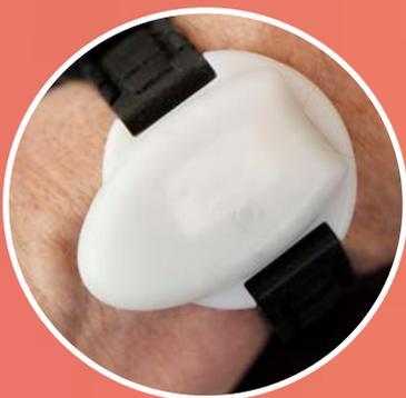
Like the Epi Care, the Epi Care mobile offers the wearer seizure management when out and about in the community. The wrist worn sensor is programmed into a mobile phone and is designed to send an alert to a dedicated number if seizure activity is detected. The sensor needs just an hour to charge and is suitable for anyone over the age of 10, making this a great choice for people wanting to manage seizure activity when accessing the community.
