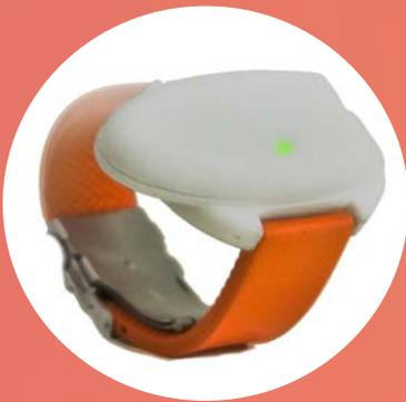
This wrist worn sensor offers increased independence compared to the epilepsy sensors often found on a bed. It is designed to detect a seizure with vigorous activity, such as a tonic-clonic seizure, and sends an alert through to a Carephone or Info Pager. Perfect for managing seizures whilst at home, day and night!
